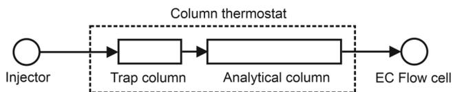
Fig 1. Column configuration.
